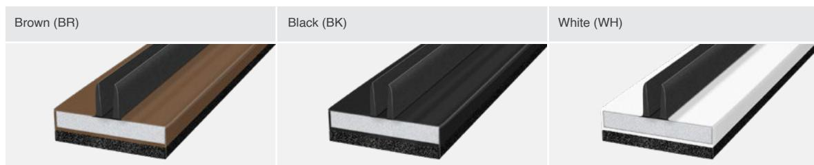
Halspan fire seals are PVC encapsulated in a range of colours shown above. Any RAL colour can be supplied subject to special order. Halspan H30 & H60 seals are sodium silicate and graphite based.
